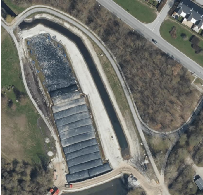
Figure 2. Dredging of sediment can take place in so-called Geotubes. Edited from envidan.com .
